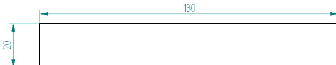
Fig.5: Standard Flexural Test Specimen Dimensions as per ASTM D - 2344
